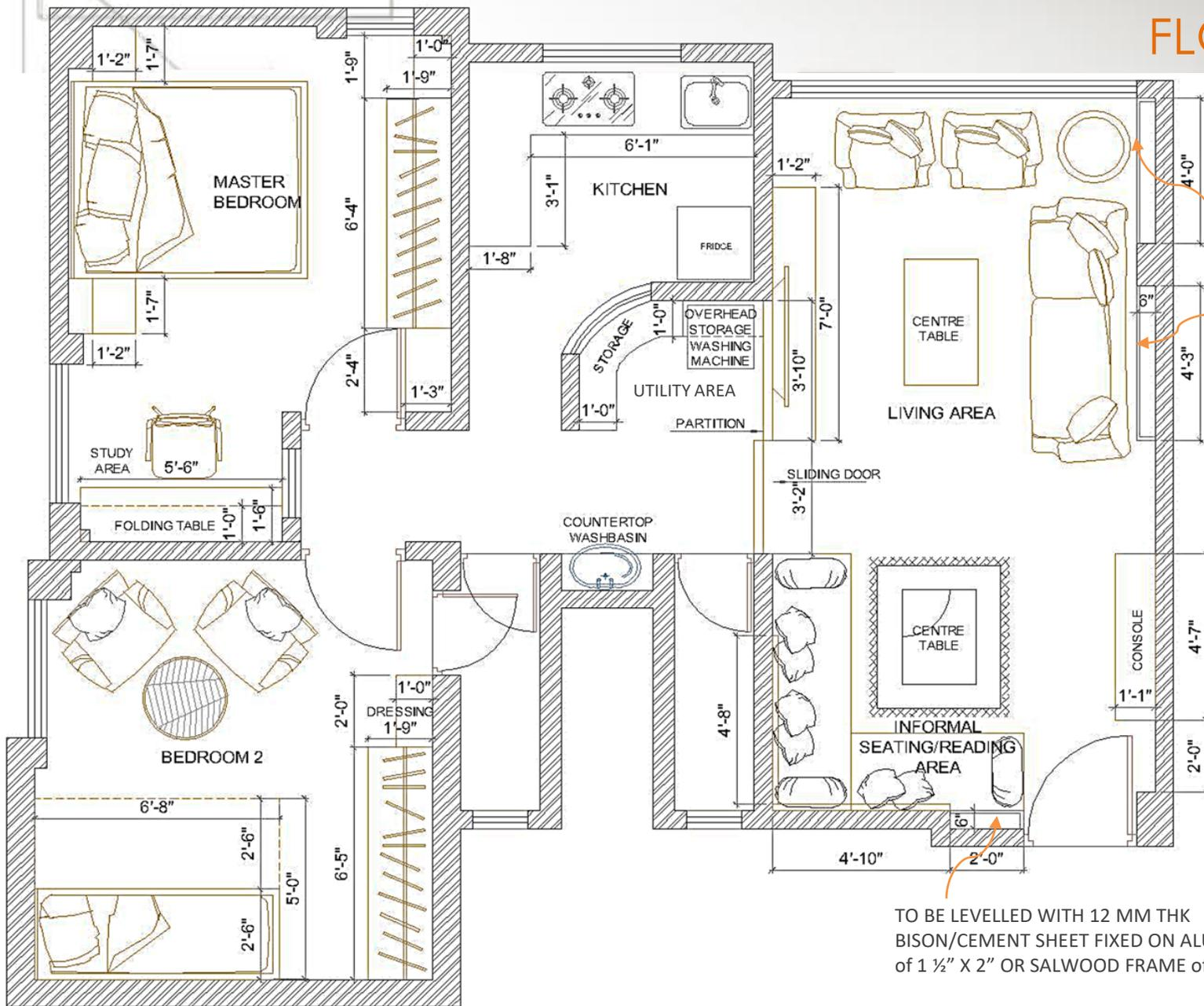
TO BE LEVELLED WITH 12 MM THK BISON/CEMENT SHEET FIXED ON ALU. FRAME OF 1 1/2" X 2" OR SALWOOD FRAME OF 1 1/2" X 2"
